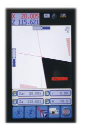
Autotargeting measurement: the viewed profile of the geometrical entities are automatically detected. The values of radii, angles, X and Z axes can be stored and/or printed on the label
