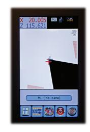
Automatic cutting edge measure. After having found the central position by means of focus bars, on the axes counters the measurement is shown without additional operations
