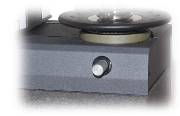
Spindle rotation brake is provided with an adjustable clutch
