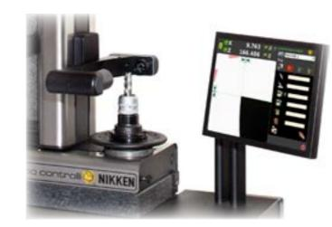
Large 15" touch screen for the best visualization of the tools and simple management functions to operate the measuring machine.
