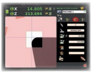
New electronic control: a powerful fanless PC with Linux operating system for the integrated management of the functions of measurement / inspection tools, machine origins and toolsets. Ease of use thanks to the integrated touch screen.
