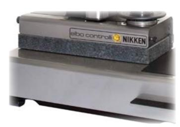
Base and column made of ground granite. The thermal inertia of this material allows the machine to be placed directly in the workshop.
