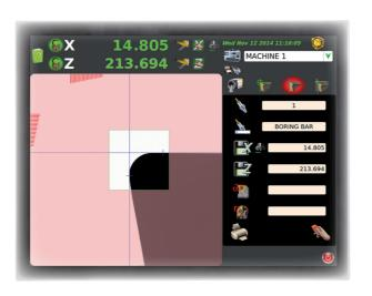
New electronic control: a powerful fanless PC with Linux operating system for the integrated management of the functions of measurement / inspection tools, machine origins and toolsets.
