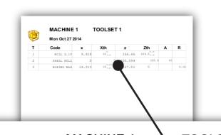
It's possible to generate and / or print a report with the theoretical values, tolerances and measurements of the selected tool table.
