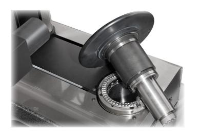
Interchangeable rotating spindle with mechanical rotation brake.
