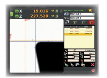
Td SIX is a new software function developed by Elbo Controlli, used to acquire tool's measurements, to input them into the tooling tables and create a file including tools offstes.
