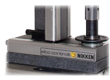
Base and column made of ground granite. The thermal inertia of this material allows the machine to be placed directly in the workshop. Mechanical elements manufactured from stainless steel.
