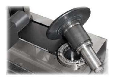
Interchangeable rotating spindle with mechanical rotation brake. Two preloaded ball cages allow a concentricity accuracy within 2 µm.
