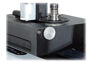
Micrometric movement of the axes are made, for the X axis with two wheels on the right and left of the machine, for the Z axis with one placed at the base of the column. This precise micrometric adjustment is indispensable for the final collimation of the cutting edge of the tools.
