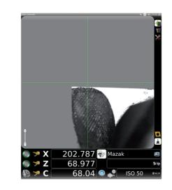
The presetter E46L is equipped with a 22" capacitive touch-screen monitor, mounted vertically for easy viewing. The screen layout and design is split into two distinct sections. The upper half of the display shows visible images of the current tool and profile. The lower half shows and allows access to all the current software functions. The operation is very intuitive and logical to allow the operator to interact with the machine and software without having to attend complex trainings sessions.
