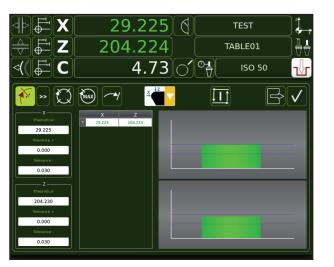
**Autofocus** function: automatic search and measurement for single edged tools.
