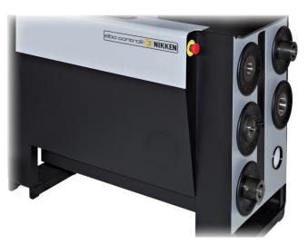
Great attention has been paid to the size and strength of the machine base which is totally produced from structural steel and is welded with both TIG and continuous welding. This concept allows the whole machine a very high stiffness the result of which guarantees high accuracy and rigidity.
