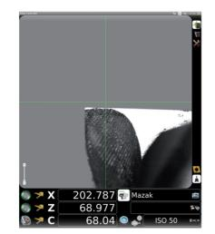
New electronics: a powerful PC running Ubuntu 14,04 LTS for the integrated management and control of the all the functions of measurement/tool inspection, machine origins and tool tables. Ease of use thanks to the integrated touch-screen.
