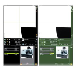
The new software provided the operator the choice of two different graphical layouts: the first provides icons similar to ISO 7000 and the second allows the familiar 'ELBO CONTROLLI' graphical interface.
