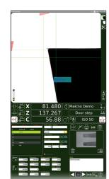
Also included for the first time is the capability for multi-measurement directly on the screen. So during tool inspection it is possible to make more than one measurement at a time on the same tool profile.
