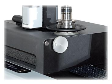
Micrometric movement of the axes are made, for the X axis with two wheels on the right and left of the machine, for the Z axis with one placed at the base of the column. This precise micrometric adjustment is indispensable for the final collimation of the cutting edge of the tools.
