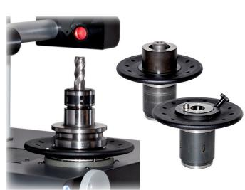
The rotating spindle is interchangeable with cartridges available for all types of machine tapers: HSK, ISO, VDI, BT, CAPTO, etc. ISO/BT spindles feature automatic tool clamping. Within the base, to the right side of the presetter spindle storage is provided for up to six cartridges. To the left also incoporated are practical shelves for additional storage capability.
