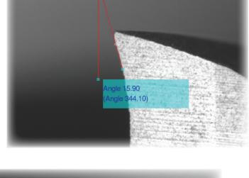
edges, diameter 10mm. Front view: front extent rake (rake angle) determines the performance of tool's working conditions.
