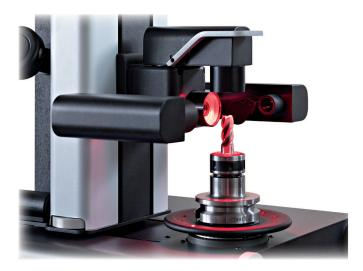
The new E46LTW is equipped with *3 cameras for the front view and* side view of the tool. The system allows to tool manufacturers and tool regrinders to measure all the geometrical features of the tool.
