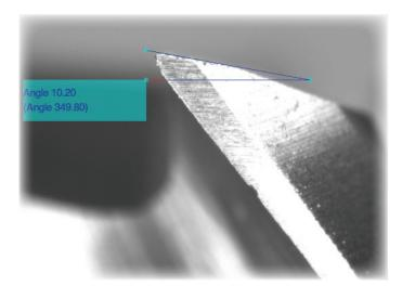
Cylindrical cutter with 4 cutting edges, diameter 6mm. Side view (chest): measure the propeller screw angle and rake angle, important to determinate to suit the type of application and the type of material being processed.
