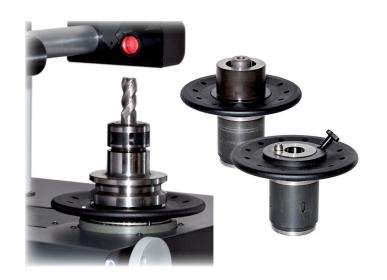
The rotating spindle is interchangeable with cartridges available for all types of machine tapers: HSK, ISO, VDI, BT, CAPTO, etc. ISO/BT spindles feature automatic tool clamping. Within the base, to the right side of the presetter spindle storage is provided for up to six cartridges. To the left also incoporated are practical shelves for additional storage capability.
