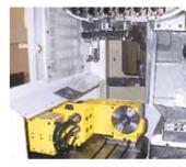
2 units of CNC rotary tables are used on the TAPPING CENTER with swing type pallet changer.
