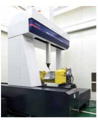
5AX Tilting Rotary Table on 3 Dimensional Measuring Machine
