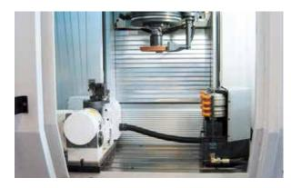
**5AX-150** for 4th and 5th axes tilting rotary table on special grinding center
