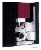
Utilization for 4th and 5th axis rotary table of the M/C for die molding
