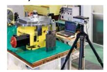
Indexing Accuracy Measurement by Laser
