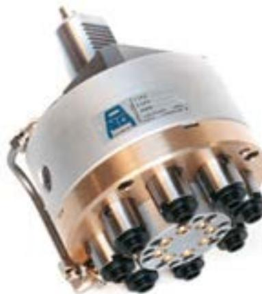
*The MT system is for small centre distances and low torque requirements. The minimum centre distance is 10 mm; below this heads reliability becomes questionable. MT units are normally very compact and with 3 or 4 spindles weigh little - 2 kg for example - and are permanent grease lubricated. Rotating*
